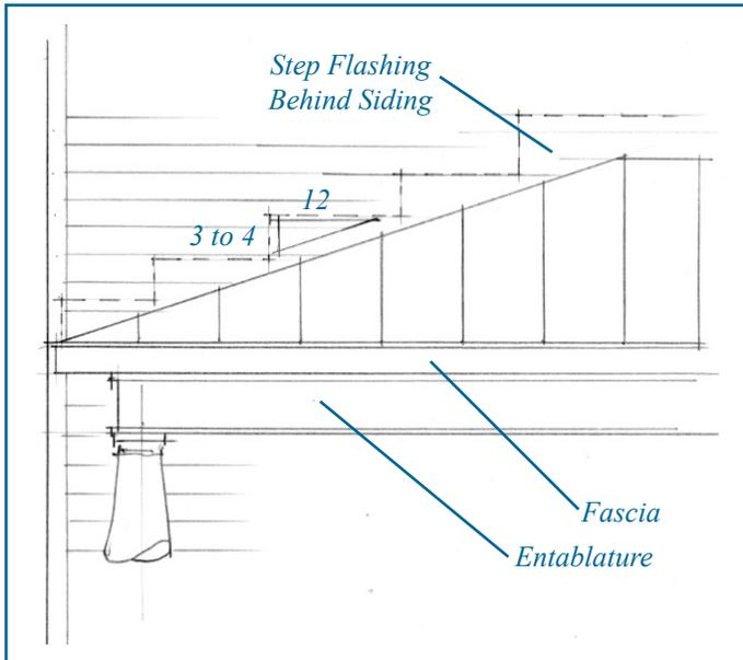
Figure 1: Front Elevation of a Hipped Porch Roof
