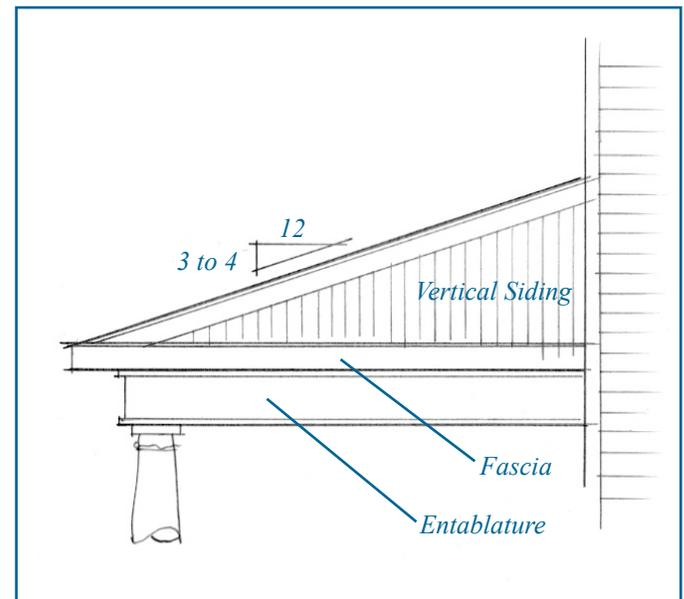
Figure 4: Side Elevation of a Shed Porch Roof
