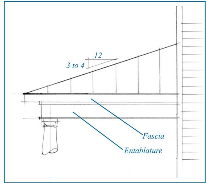
Figure 2: Side Elevation of a Hipped Porch Roof
