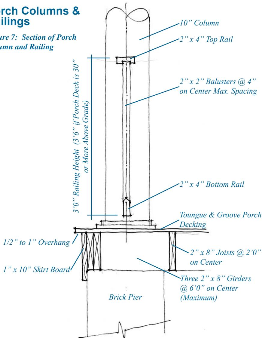
The porch *columns* provide the support for the porch roof beam (*entablature*), which supports the roof structure. Seen as decorative elements of the porch assembly, they take on many forms, from the smooth round Doric columns to the fluted round Corinthian columns with elaborate *capitals* to the intricate *turned wood* columns, to the tapered square box columns. They extend from the entablature to the porch deck and are supported by the porch deck beam below the porch deck.
