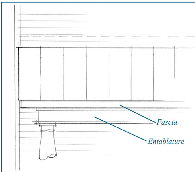
Figure 3: Front Elevation of a Shed Porch Roof
